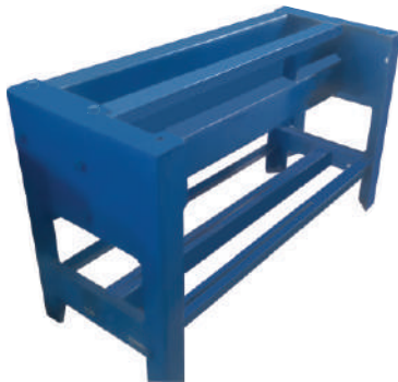
IGD05/10 TALL BED PLATE (With Deflector Sheave mounting arrangement)
